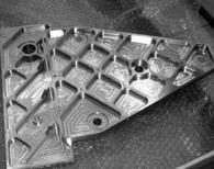
■ Finished rear surface. Differing wall thickness and pocket variations breaks up vibration
