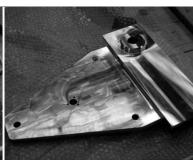
■ The Keel is diamond machined for the smoothest finish possible
